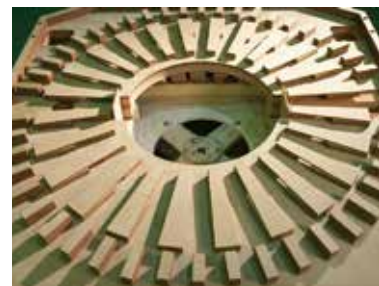
油道結構 Construction of Oil Duct
